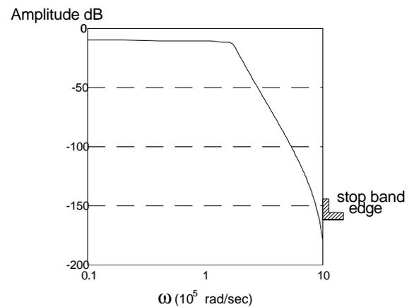
Figure 3 (a) Response of Genetically derived LC ladder filter with no parasitics considered.
