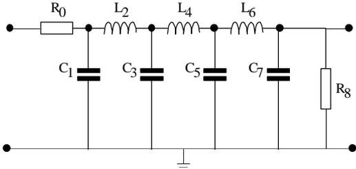
Figure 1 Low Pass All-Pole Ladder Structure
